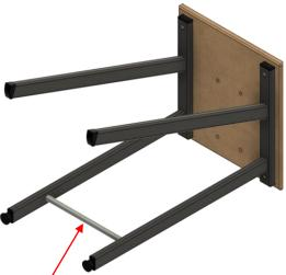
Now fit the brace bars between the rear leg using the M8 x 40mm bolts and washers.
