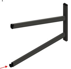
Screw the M10 nuts (item 13) all the way onto the threads of the adjustable feet (item no. 4), then screw the feet into the threaded hole on the bottom of each of the rear legs. When fully assembled these feet can be adjusted to level the bench, and the nuts lock them in place.
