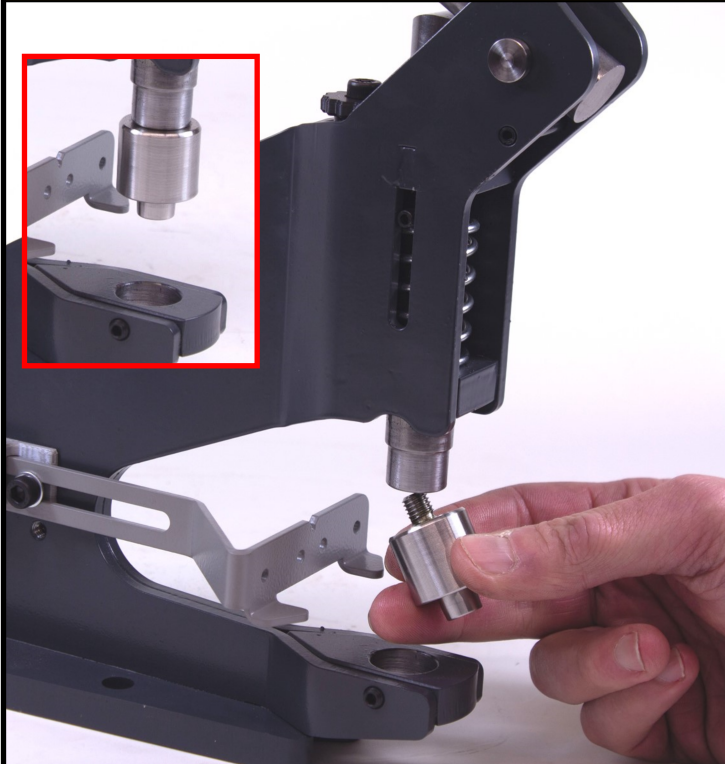
Step 1. Screw the top die into the underside of the vertical rod.
