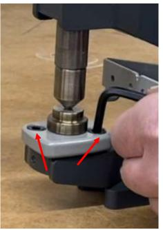
Step 5. Holding the dies in position retighten the 2 DAP screws to fix the lower die in to a central position in relation to the top die.
