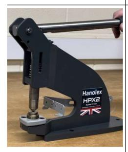
Step 4. Applying light pressure to the handle to lower the top die down so its tip enters the hole in the lower die. As
