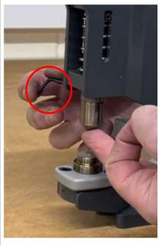
Step 3. Insert the top cutter into movable shaft and tighten the retaining screw.
