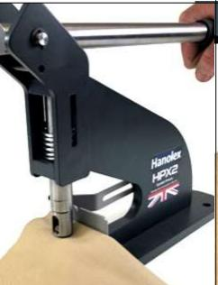
Step 5. Now lower the top die again and apply firm pressure to set the eyelet.
