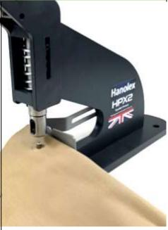
Step 3. Lift up the die, the pin will now be protruding through the material. The waste material is ejected through the slot in the top die.
