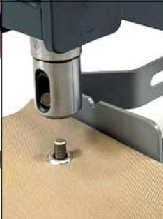
Step 6. When you lift the top die clear the fitted eyelet will be sat on the lower die and can be removed from the die and the operation repeated.
