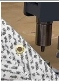
Step 6. lower the top die and apply pressure to set the eyelet, for larger eyelets remember the press applies the most pressure when the handle is almost horizontal.
