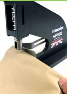
Step 2. Place the material between the dies where you want to fit the eyelet.
