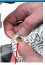
Step 3. Inset the barrel of the eyelet into the hole in the material, add a washer (if used) over the barrel on the back of the material.
