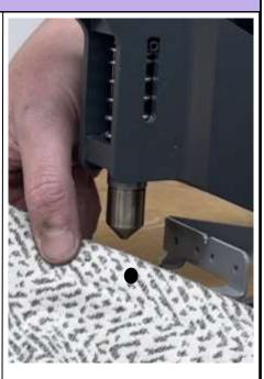
Step 3. lift the die to reveal the cut hole. Repeat as required.
