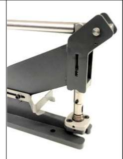
Step 6. Carefully lower the shaft down onto the spigot of the top die. Move the lower die adjustment plate to allow the dies to centralise with the shaft.
