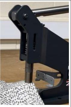
Step 5. lower the top die and apply pressure to set the eyelet, for larger eyelets remember the press applies the most pressure when the handle is almost horizontal.
