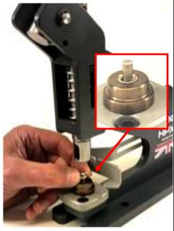
Step 1. Place a flat ring over the pin on the lower die so it sits in the recess.
