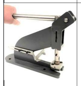
Step 4. Check that the dies are aligned by lowering the top die on to the lower die. It should lower smoothly without the dies catching on each other. If they do catch repeat the previous steps. PLEASE NOTE IF THE DIES CATCH THEY CAN EASILY BECOME DAMAGED.
