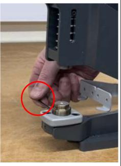
Step 2. Insert the lower cutting die into the hole in the DAP and tighten the locking screw.
