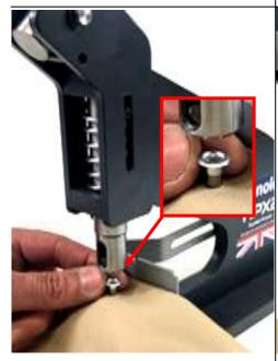
Step 4. Place an eyelet on the pin protruding through the material (note the correct way round)
