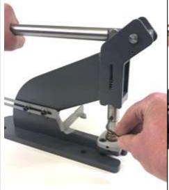
Step 7. Keeping the dies together tighten the top die retaining screw.
