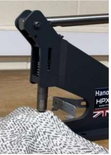
Step 2. lower the top die down and touch the material, then continue to apply pressure until you hear and feel a click as the material is cut.
