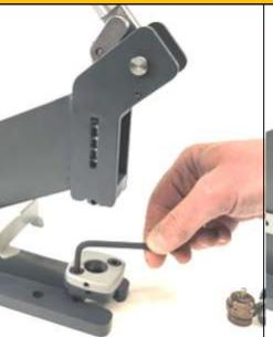
Step 2. Using the 5mm hexagon key loosen the two screws on the lower die adjustment plate.
