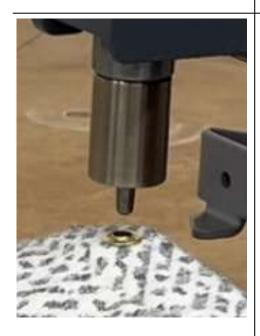
Step 4. with the eyelet side to the bottom and the washer side to the top place them on the lower die.
