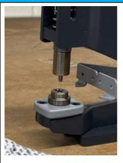
Step 2. Fit the setting dies into the press, as the DAP has already been aligned this should not need adjusting. Be carful not to mix the cutting and setting dies together.
