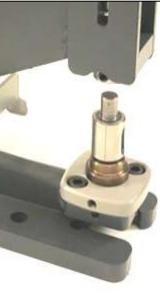
Step 5. Next, place the top die onto the lower die as above.
