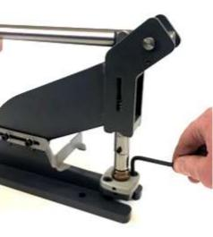
Step 8. Then tighten the two screws on the lower die adjustment plate.
