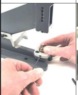
Step 4. Insert the lower die in to the lower die adjustment plate and fasten in place using the 3mm hexagon key to tighten the screw on the side.
