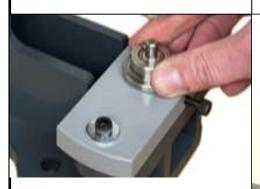
Step 4. Insert the lower die in to the lower die adjustment plate and fasten in place using the 3mm hexagon key to tighten the screw on the side.
