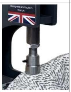
Step 5. lower the top die and apply pressure to set the eyelet, for larger eyelets remember the press applies the most pressure when the handle is almost horizontal.
