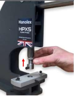
Step 2. Loosen the upper die holder (UDH) this is done by loosening the locking nut with the supplied spanner. Then screw the UDH up in to the machines shaft.
