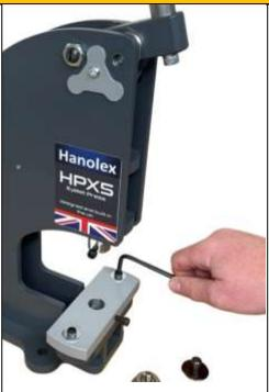
Step 2. Using the 5mm hexagon key loosen the two screws on the lower die adjustment plate.
