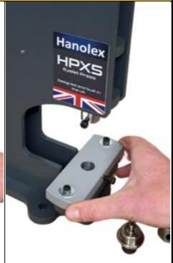
Step 3. This will allow the lower die adjustment plate to move a few millimeters in all directions.
