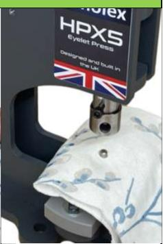
Step 3. Lift up the die, the pin will now be protruding through the material. The waste material is ejected through the slot in the top die.
