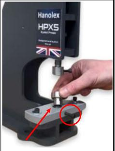
Step 3. Insert the lower cutting die into the hole in the DAP and tighten the locking screw.
