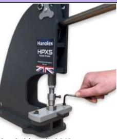
Step 9. tighten the 2 DAP screws. Then lift the handle up to raise the top die clear, the dies are now ready to be used.
