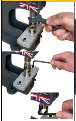
Step 7. Before lifting the handle, tighten the locking nut, the 2 Die adjustment plate screws AND the screw that holds the top die on the top die.
