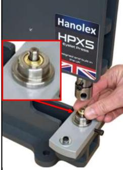
Combination or "combi" eyelet dies first cut the material with the first pull of the handle and then set the eyelets with a second pull.
