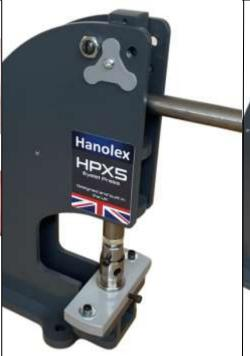
Step 8. Check that the dies are correctly aligned by lifting then lowering the top die on to the lower die. It should lower smoothly without the dies catching on each other. If they do catch repeat the previous steps. PLEASE NOTE IF THE DIES CATCH THEY CAN EASILY BECOME DAMAGED.
