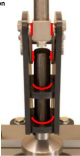
To ensure accuracy and long life the shaft and mechanism of the press should be oiled on a regular basis .
