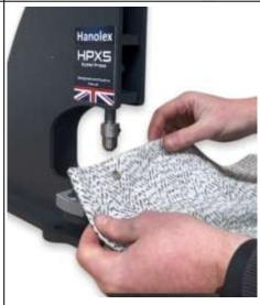
Step 12. lift the die to reveal the cut hole. Repeat as required.
