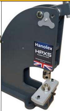
Step 9. When you are satisfied that there is no catching, Lift the handle up and the machine is now ready to use with the combination dies.
