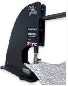
Step 11. lower the top die down and touch the material, then continue to apply pressure until you hear and feel a click as the material is cut.
