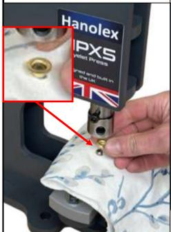
Step 4. Place an eyelet on the pin protruding through the material (note the correct way round)
