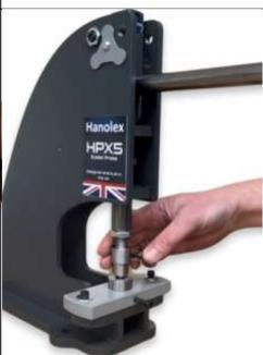
Step 5. Lower the handle down to the horizontal position then screw the TDH containing the top die down so it touches the lower die and wont move any further. As you lower the top die ensure the lower die is centralised around it.
