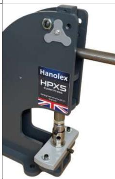
Step 6. Carefully pull the handle and lower the machine shaft down onto the spigot of the top die so the handle is horizontal. Screw the top die holder down so the die spigot fully engages in it
