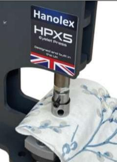
Step 5. Now lower the top die again and apply firm pressure to set the eyelet.
