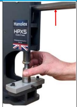
Step 2. if required adjust the upper die holder UDH to allow the handle to sit horizontally when the dies are together
