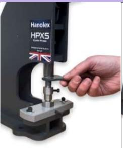
Step 8. lock the TDH in place by tightening the locking nut up against the machine shaft.
