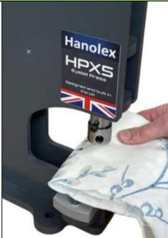
Step 2. Place the material between the dies where you want to fit the eyelet. Lower the top die down and apply firm pressure to cut the hole in the material.
