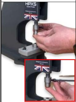
Step 4. Insert the top cutter into the top die holder (TDH) and tighten the retaining screw.
