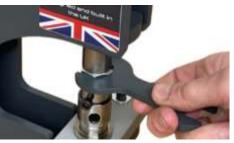
Loosen the locking nut on the shaft with the supplied spanner to free up the top die holder.
