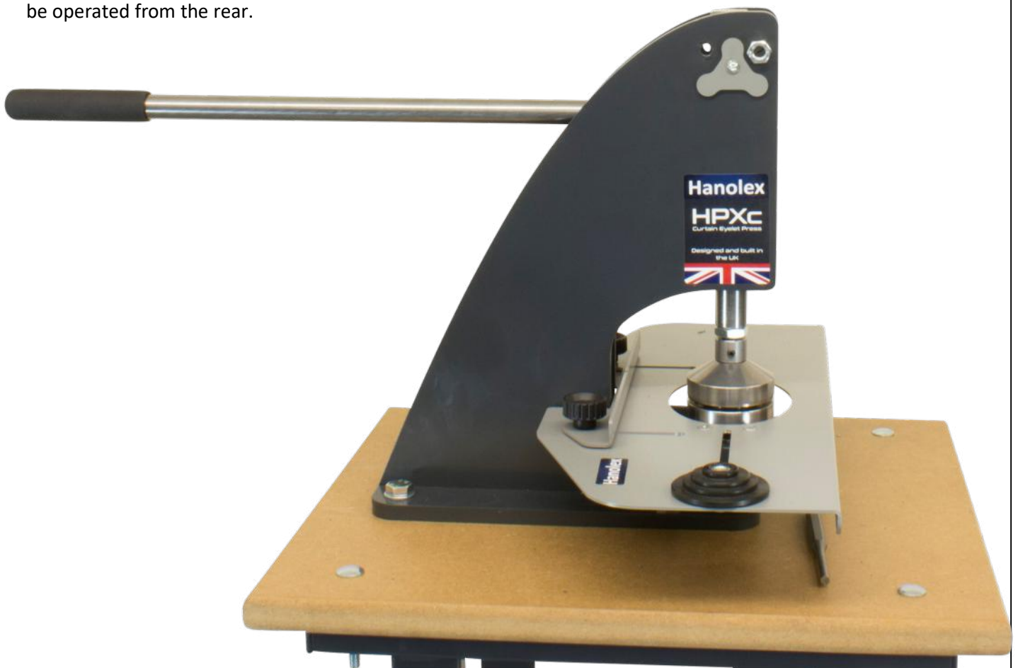
Fig 4 Below shows the HPXc press set up to be operated from the rear.
