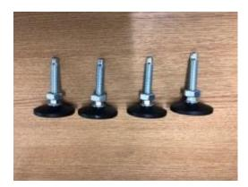
Step 1 - Screw Locking Nuts on to thread.
