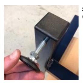
Step 2 - Screw in to threaded hole on underside of frame.
